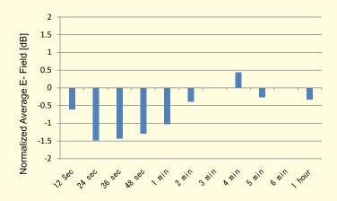
Fig. 6. Time average E-fields of base station 2 normalized to the value of the 6 minutes measurement time.
