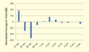
Fig. 5. Time average E-fields of base station 1 normalized to the value of the 6 minutes measurement time.
